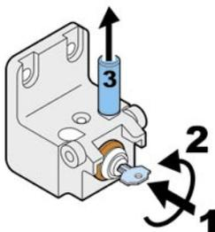
Insert key **1**, turn **2**, and remove pin **3**.
