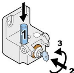
Insert pin **1**, insert key **2** and turn **3**.
