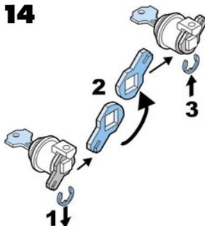
Remove door latch **1**, turn over **2** and reassemble **3**.
